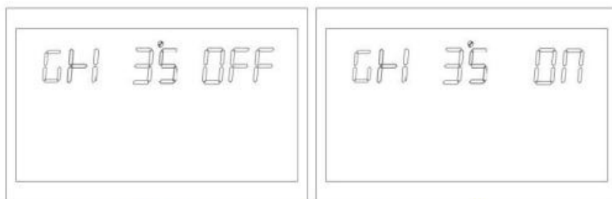
Figure 1-43 Grid-connected inverter function setting page
