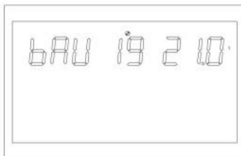
Figure 1-29 Setting the battery shutdown point
