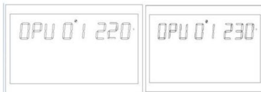
Figure 1-12 Setting the output voltage
