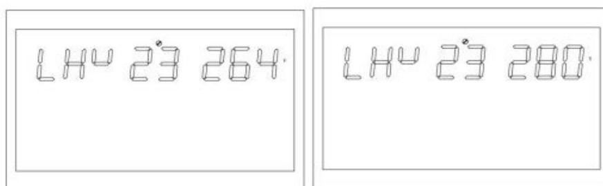
Figure 1-33 Setting high voltage point of grid
