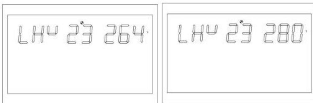
Figure 1-33 Setting high voltage point of grid
