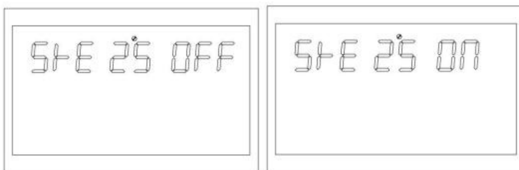
Figure 1-35 Setting the soft startup of the inverter
