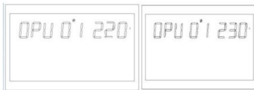
Figure 1-12 Setting the output voltage
